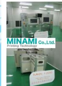
Solder Printer Ball Placer (8~12 inch. Wafer)
